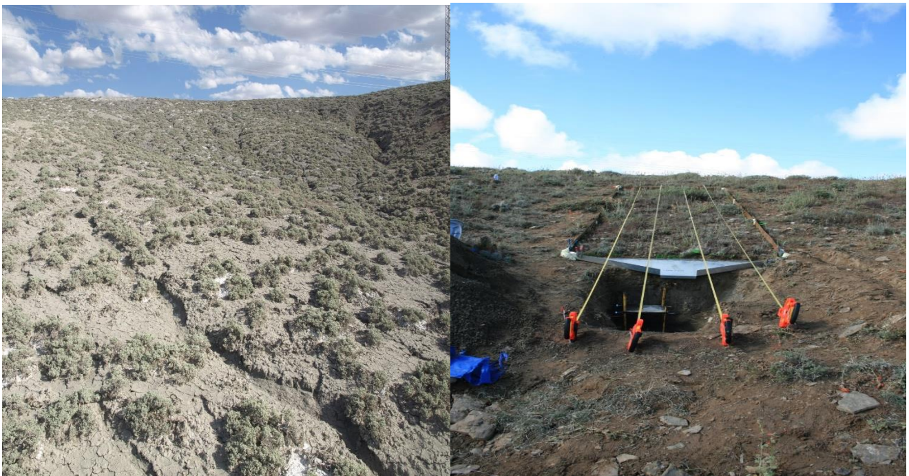
Figure 15. Sparse vegetation at Dry X illustrating concentrated flow and formation of gullies due to limited vegetation and inter-connected interspaces (left) and measuring tapes for determine vegetation gap, rill density and canopy and ground cover (right).
