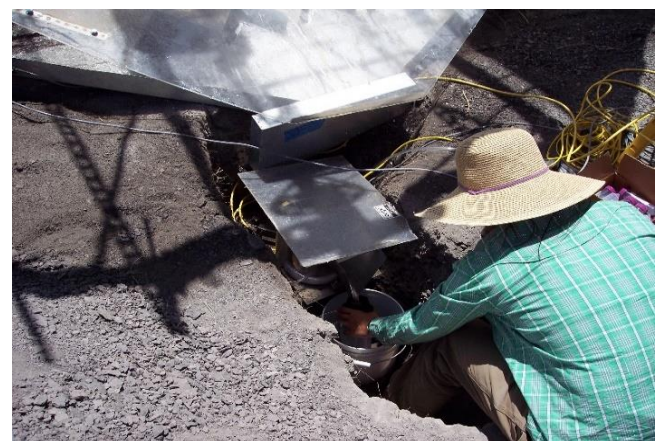
Figure 6. Measuring timed-sampling of concentration to steady state runoff rate (left) and runoff water quality (right).
