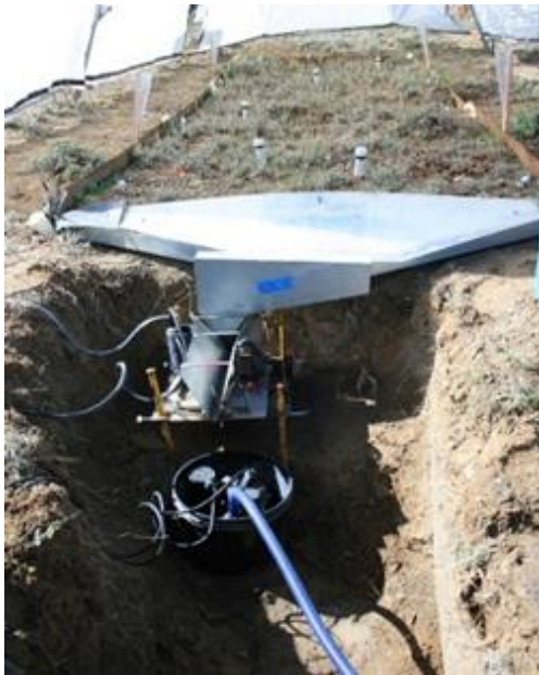
Figure 30. Super critical flume for measuring runoff volume, flow rates runoff, sediment concentration, and water quality (left) and collecting water quality samples to determine salt transport off site (right). Detailed photos showing all steps in data collection are in appendix II.
