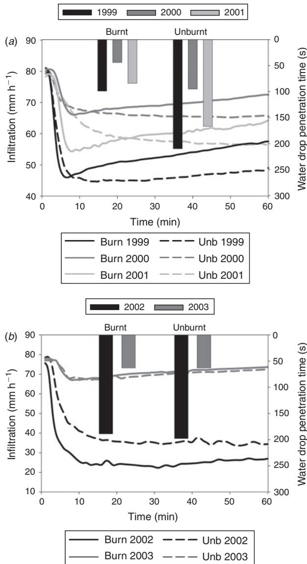
**Fig. 4.** Infiltration of simulated rainfall ( $85\text{-mm}\cdot\text{h}^{-1}$  intensity) and strength of soil water repellency (measured as water drop penetration time, WDPT) on sagebrush rangeland in Nevada, USA (a) (Pierson *et al.* 2008a, 2008b) and Idaho, USA (b) (Pierson *et al.* 2009).
