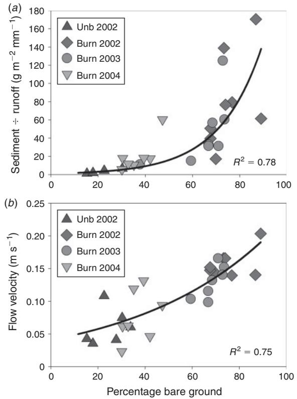
**Fig. 5.** Sediment yield per unit of runoff (a) and velocity of concentrated flow (b) compared with bare ground measured for rainfall simulation plots ( $32.5\text{ m}^2$ ,  $85\text{ mm}\cdot\text{h}^{-1}$ , 60 min) and overland flow experiments ( $12\text{ L}\cdot\text{min}^{-1}$ ) respectively on burnt (Burn) and unburnt (Unb) areas of sagebrush rangeland immediately (2002), and 1 (2003) and 2 (2004) years after fire. Data from Pierson *et al.* (2009).
